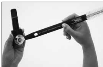
CLEANING THE PRESSURE REGULATOR
